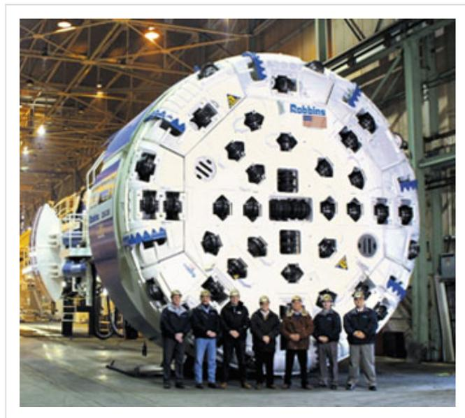
**TBM cutterhead for Kárahnjúkar, Iceland**
