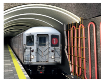
Turning underground metro lines into heat-recovery systems
