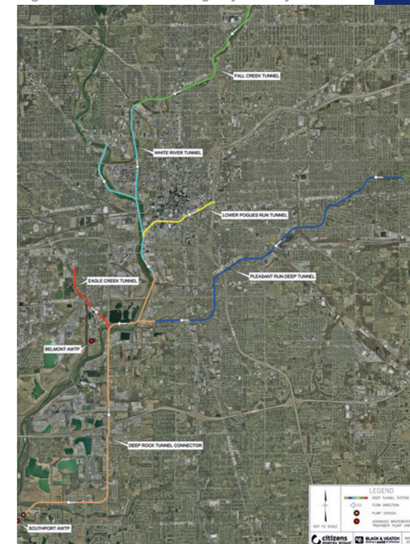
Fig 1. Six sections of the DigIndy CSO system
