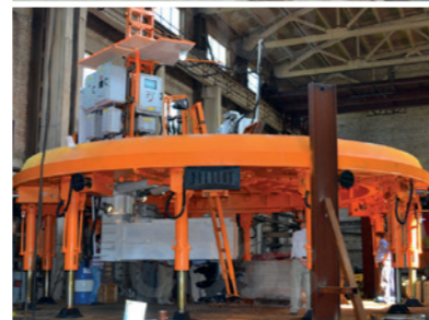
Above: Portal of the dual carriageway infrastructure Below: 1SPKV-8.0 shaft sinking machine used on earlier Ufa tunnel works
