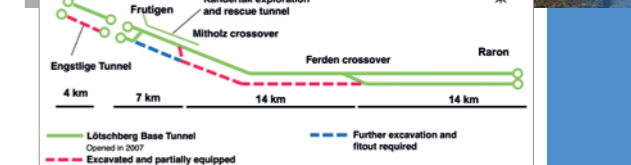
Fig 1. Operating tunnel and completion works
