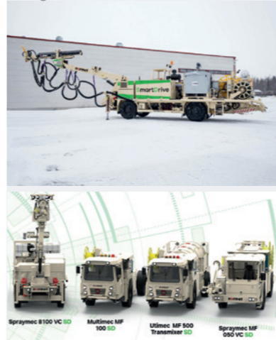
From top: SmartSpray SmartDrive shotcreting from Normet ; Part of the range of new SmartDrive machines
