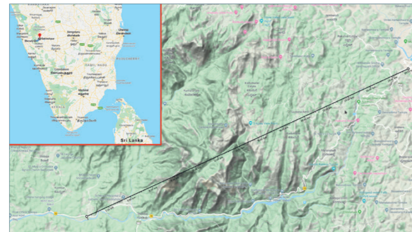
Fig 1. Proposed Western Ghats underpass: the road tunnel of 29km being considered will be challenging work due to the elevation differences and the prevailing geology. It has been discussed for some time and perhaps this decade is the decade in which it will advance
