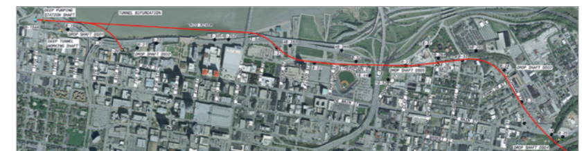
Fig 1. The 2.5 mile route cuts under the Ohio River and eliminates four storage basins
